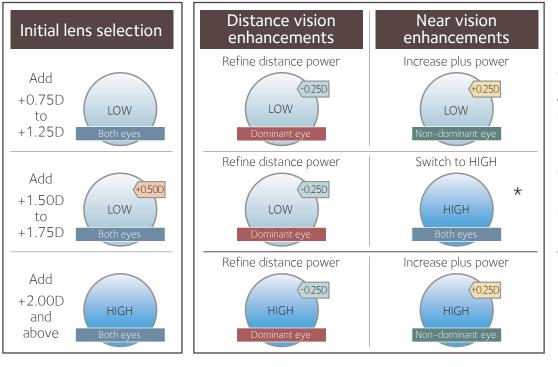
General tip: Always push the plus giving the least reading Add needed. For enhancements use full aperture trial lenses increasing the power as needed. Binocular adjustments are also possible.
